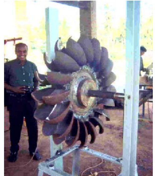
Microhydro-turbine for village cooperative/society, Sri Lanka. Photo: ITDG/Practical Solutions
